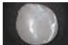
**fig. 4 and fig. 5** Enlargements of fig. 3 showing clear porcelain fully vitrified (left) and non-vitrified or under-processed (right).
